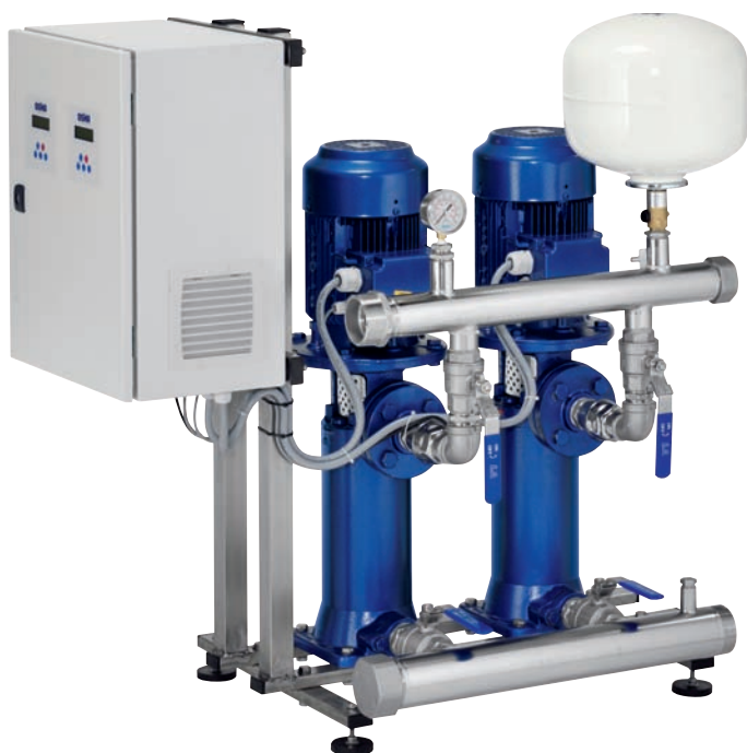
System with two high pressure centrifugal pumps type CVP. Each motor is operated by a frequency controller inside the electronic control box. Systems with up to 4 pumps are available quickly due to the modular construction. The shown system is a special construction, equipped with additional gate valves and a pressure gauge on discharge side.
