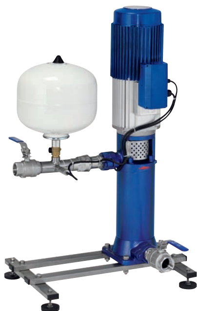
System with one pump, including motor type MAI with integrated frequency controller (up to 4 kW). Delivery includes the required sensor.
